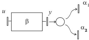
Fig. 4. A system with two divergent outputs.
