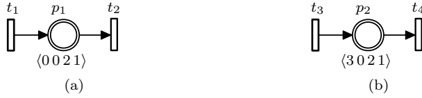
Figure 2: In (a) \mathcal{H}_1 = \langle 0 \ 0 \ 2 \ 1 \rangle satisfies the FIFO condition. In (b) \mathcal{H}_2 = \langle 3 \ 0 \ 2 \ 1 \rangle violates the FIFO condition.
