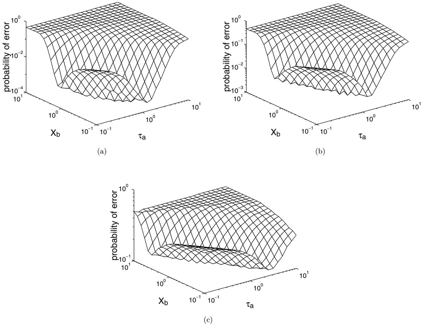
Fig. 2. Quantitative influence of the nonlinear filter parameters  $\tau_a$  and  $X_b$  on the probability of detection error  $P_{er}$  of Eq. (3), for different noise power densities  $D$ . The results are obtained by Monte Carlo simulations. (a)  $D = 0.0275$ . (b)  $D = 0.0524$ . (c)  $D = 0.304$ .
