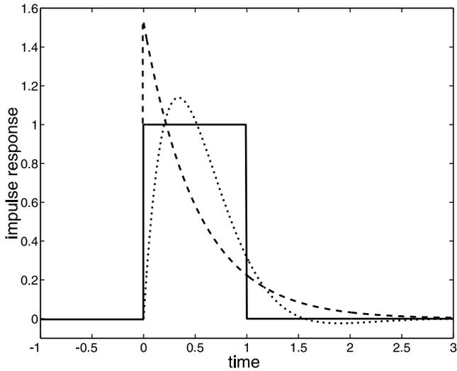
Fig. 5. Impulse response  $h''(t)$  of the closest approximation of the matched filter by a first- and second-order linear filter with no zeroes. Solid line represents the impulse response of the ideal matched filter  $h(t)$ , dotted line stands for the first-order filter and dashed line for the second-order filter.  $T_p$  and  $A$  are taken equal to unity.
