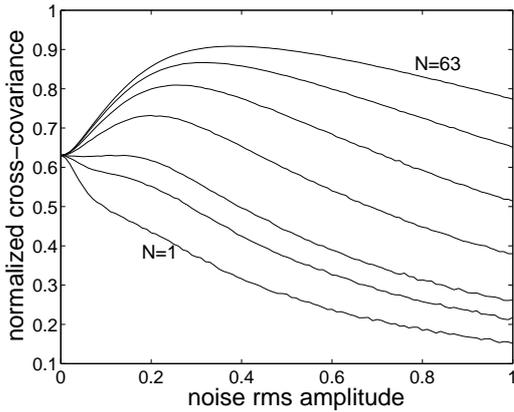
Figure 3: Normalized cross-covariance of original “lena” image correctly exposed with the image transmitted by the process of Eq. (3) as a function of the level of the noise  $\sigma_\eta$  for various number of acquisitions  $N = 1, 2, 3, 7, 15, 31, 63$ . The exposure parameter  $k_{ex} = 0.75$  is the same as in Figure 2.
