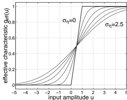
Figure 1: Effective input–output characteristic  $g_{\text{eff}}(\cdot)$  of Eq. (2) for the device of Eq. (7) in presence of Gaussian centered noise with various rms amplitude  $\sigma_\eta = 0, 0.5, 1, 1.5, 2, 2.5$ .
