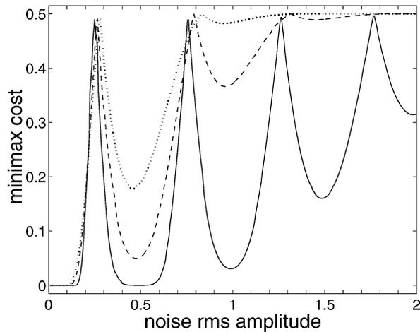
Fig. 8. Minimax cost  $C_{\text{minimax}}$  of Eq. (8) of the optimal minimax detector, as a function of the rms amplitude  $\sigma_\eta$  of the Gaussian-mixture noise  $\eta(t)$  with  $m = 0.9$  (dotted line),  $m = 0.95$  (dashed line),  $m = 0.99$  (solid line). Also  $C_{00} = C_{11} = 0$ ,  $C_{01} = C_{10} = 1$ ,  $\nu_0 = 1$ ,  $\nu_1 = 2/3$ , with  $N = 11$  data samples equispaced with time step 0.2 from  $t_1 = 0$  to  $t_{11} = 2$ .
