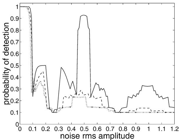
Fig. 6. Probability of detection  $P_d$  of Eq. (5) of the optimal Neyman–Pearson detector, as a function of the rms amplitude  $\sigma_\eta$  of the Gaussian-mixture noise  $\eta(t)$  with  $m = 0.9$  (dotted line),  $m = 0.95$  (dashed line),  $m = 0.99$  (solid line). Also  $P_{f,\text{sup}} = 0.1$ ,  $\nu_0 = 1$ ,  $\nu_1 = 2/3$ , with  $N = 3$  data samples measured at  $t_1 = 0.1$ ,  $t_2 = 0.4$ , and  $t_3 = 0.6$ .
