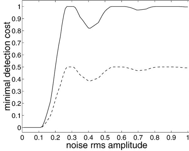
Fig. 1. Minimal detection cost  $C_{\min}$  from Eq. (19) of the optimal Bayesian detector, as a function of the rms amplitude  $\sigma_\eta$  of the zero-mean uniform noise  $\eta(t)$ . Also  $C_{00} = C_{11} = 0$ ,  $P_0 = 0.5$ ,  $\nu_0 = 1$ ,  $\nu_1 = 2/3$ , with  $N = 13$  data samples equispaced with time step 0.2 from  $t_1 = 0$  to  $t_{13} = 2.4$ . Solid line:  $C_{10} = 2$  and  $C_{01} = 5$ , dashed line:  $C_{10} = 1$  and  $C_{01} = 2$ .
