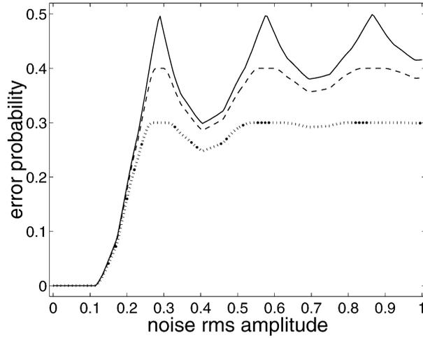
Fig. 3. Probability of detection error  $P_{er}$  from Eq. (19) of the optimal MAP detector, as a function of the rms amplitude  $\sigma_\eta$  of the zero-mean uniform noise  $\eta(t)$ . Also  $\nu_0 = 1$ ,  $\nu_1 = 2/3$ , with  $N = 11$  data samples equispaced with time step 0.2 from  $t_1 = 0$  to  $t_{11} = 2$ . Solid line:  $P_0 = 0.5$ , dashed line:  $P_0 = 0.4$ , dotted line:  $P_0 = 0.3$ .
