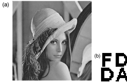
Fig. 9. (a) The marked image ‘Lena’ filtered by a high pass filter with window size 3 \times 3 . (b) The recovered binary image S^* by the isolated saturating detector. Here, \tau_a = 0.1T_b and X_b = 0.125A .
