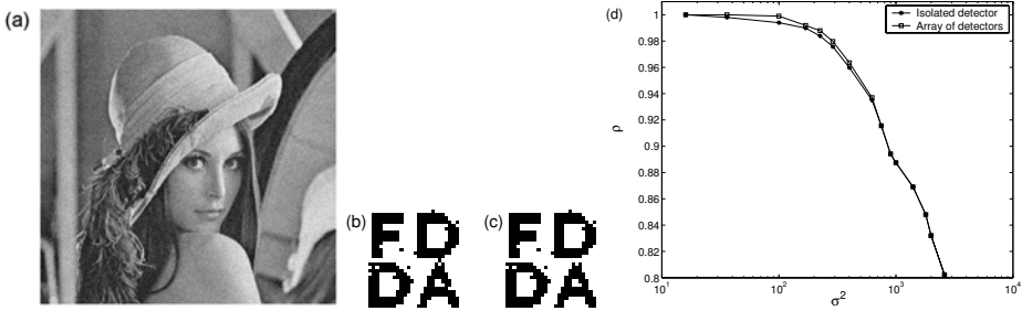
Fig. 6. (a) Watermarked image ‘Lena’ corrupted by Gaussian noise with variance \sigma^2 = 225 . (b) The recovered binary image via the isolated saturating detector, and (c) by the array of saturating detectors at the optimal noise intensity D_\eta/\Delta t = 100 . (d) Similarity \rho as a function of Gaussian noise variance \sigma^2 . Here, \tau_a = 0.1T_b , X_b = 0.25A and the array size K = 60 .
