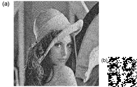
Fig. 12. (a) The marked image after dithering. (b) The recovered binary image by the isolated saturating detector. Here, \tau_a = 0.05T_b and X_b = A/4 .
