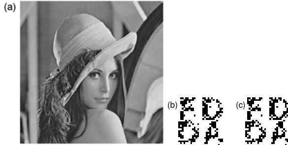
Fig. 3. (a) JPEG compressed version of the marked image ‘Lena’ with 65% quality and 0% smoothing. (b) The recovered binary image via the isolated saturating detector, and (c) the array of saturating detectors at the optimal noise intensity D_\eta/\Delta t = 5 . Here, \tau_a = 0.05T_b , X_b = 0.25A and the array size K = 60 .
