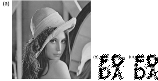
Fig. 8. (a) The marked image ‘Lena’ filtered by a low pass filter with window size 3 \times 3 . (b) The recovered binary image S^* via the isolated saturating detector, and (c) the array of saturating detectors at the optimal noise intensity D_{\eta}/\Delta t = 30 . Here, \tau_a = 0.1T_b , X_b = 0.125A and the array size K = 60 .
