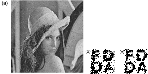
Fig. 10. (a) The marked image ‘Lena’ added by salt & pepper noise with noise density 0.05. (b) The recovered binary image S^* via the isolated saturating detector, and (c) the array of saturating detectors at the optimal noise intensity D_\eta/\Delta t = 0.5 . Here, \tau_a = 0.1T_b , X_b = A/(4\sqrt{2}) and the array size K = 60 .
