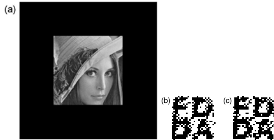
Fig. 7. (a) The marked image ‘Lena’ after cropping as a 256 \times 256 subimage. The black background indicates the cutting section. (b) The recovered binary image S^* via the isolated saturating detector and (c) the array of saturating detectors at the optimal noise intensity D_\eta/\Delta t = 300 . Here, \tau_a = 0.1T_b , X_b = 0.25A and the array size K = 60 .
