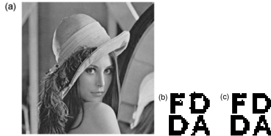
Fig. 13. (a) The marked image embedded with five different watermarks. (b) The recovered binary image S^* via the isolated saturating detector, and (c) the array of saturating detectors at the optimal noise intensity D_\eta/\Delta t = 1 . Here, \tau_a = 0.1T_b , X_b = A/4 and the array size K = 60 .
