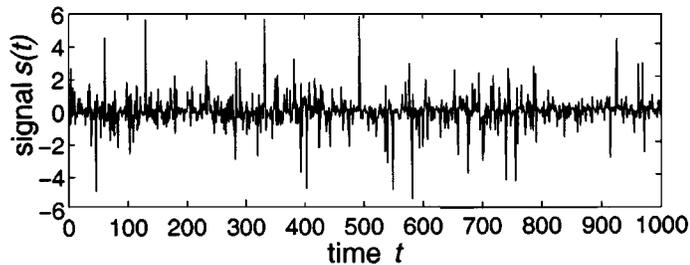
Fig. 4. Realization of a generalized Gaussian noise with exponent  $1/2$  generated with the algorithm of Fig. 2 to implement the function of (8) performing the transformation of a uniform noise.
