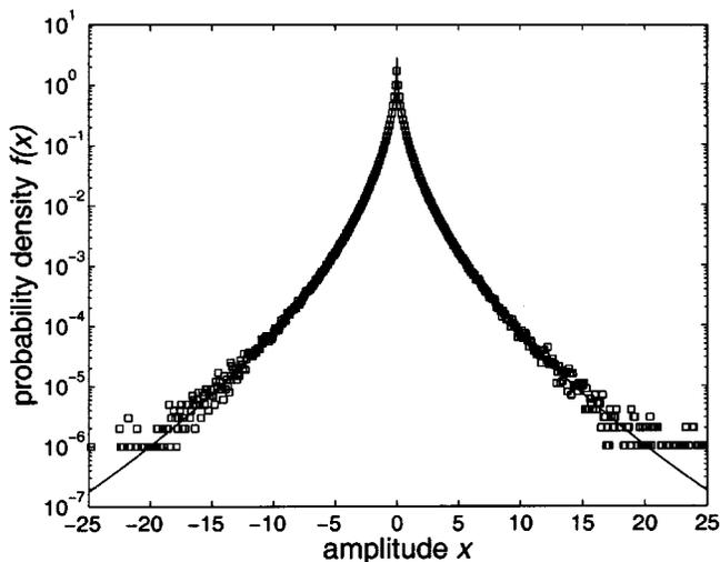
Fig. 5. Probability density function estimated for the generalized Gaussian noise with exponent  $1/2$  synthesized as in Fig. 4, superimposed to the theoretical model of (2) (continuous solid line).
