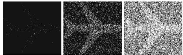
Fig. 2. Output image  $Y(u, v)$  of the hard limiter of Eq. (6) for increasing rms amplitude  $\sqrt{2}\sigma_N$  of the speckle noise  $N(u, v)$ . From left to right  $\sqrt{2}\sigma_N=0.28, 0.84$  (optimal value), 2.81; with threshold  $\theta=0.75$ ,  $p_1=0.27$  and  $\{R_0=1/2, R_1=1\}$ .
