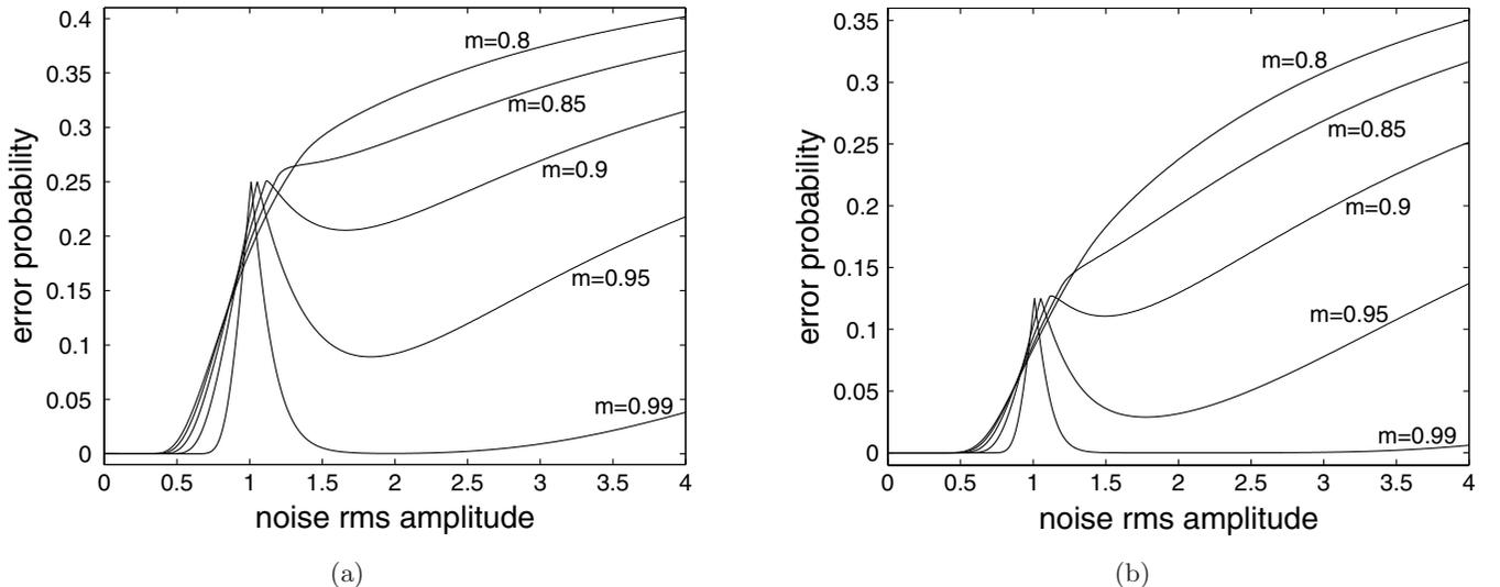
Fig. 1. Probability of error  $P_{\text{er}}$  of Eq. (7) for the optimal detector of Eq. (5), as a function of the rms amplitude  $\sigma_\eta$  of the Gaussian-mixture noise  $\eta(t)$  from Eq. (12) at different  $m$ . Also,  $s_0(t) \equiv s_0 = -1$ ,  $s_1(t) \equiv s_1 = 1$  and  $P_0 = 1/2$ ; (a)  $N = 1$  or (b)  $N = 2$ .
