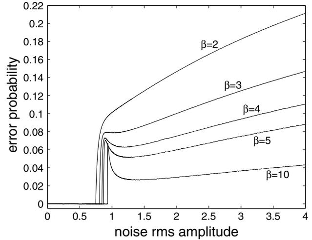
Fig. 2. Probability of error  $P_{\text{er}}$  of Eq. (7) for the optimal detector of Eq. (5), as a function of the rms amplitude  $\sigma_\eta$  of the noise  $\eta(t)$  from Eq. (15) at different  $\beta$ . Also,  $s_0(t) \equiv s_0 = -1$ ,  $s_1(t) \equiv s_1 = 1$ ,  $P_0 = 1/2$  and  $N = 1$ .
