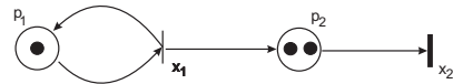
Fig. 1. Example 1: elementary P-timed Petri net with a self-loop (the observable transition is x_2 ).
