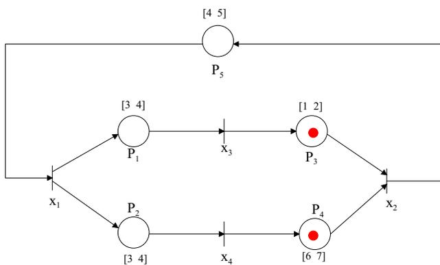
Figure 2: A p-time event graph with circuit
