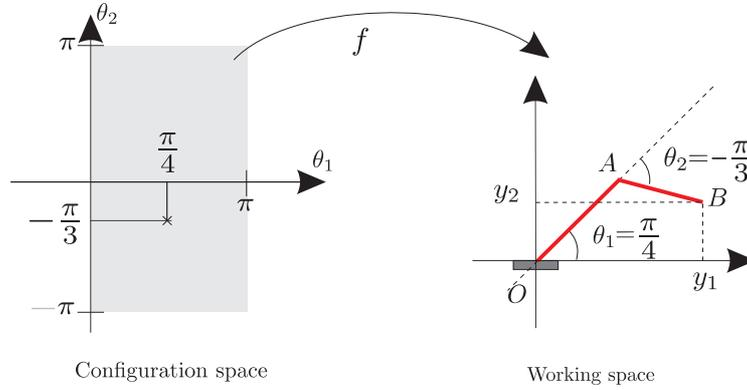
**Figure 1.1.** A point in the configuration space and its corresponding robot configuration.
