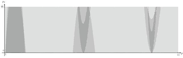
Fig. 10. Solution of the process of enclosure of \mu_{[p]} obtained by IAVIA. In light gray, the value of the parameters for which the system (53) is structurally identifiable ( \mu^+ = \mu^- = 1 ). The two dark gray zones correspond to the value of the parameters for which the system (53) is locally identifiable. 2 or 3 parameter vectors are possible ( \mu^+ = \mu^- = 2 or \mu^+ = \mu^- = 3 ). In the white domains, the injectivity function is enclosed.
