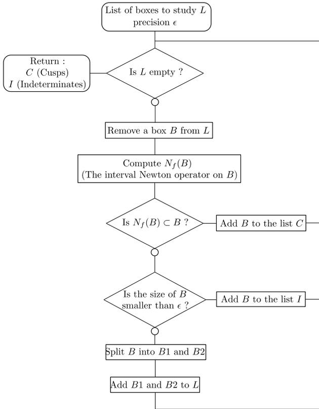
Figure 4. Interval Newton Algorithm.
