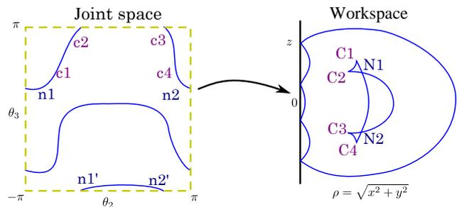
Figure 2. Singular sets in the space of the last two joints  $(\theta_2, \theta_3)$  and in the cross section  $(\rho = \sqrt{x^2 + y^2}, z)$  of the workspace, for a 3R orthogonal manipulator with parameters  $d_2 = 1, d_3 = 1.5, d_4 = 0.7, r_2 = 0.5, r_3 = 0.5$ .
