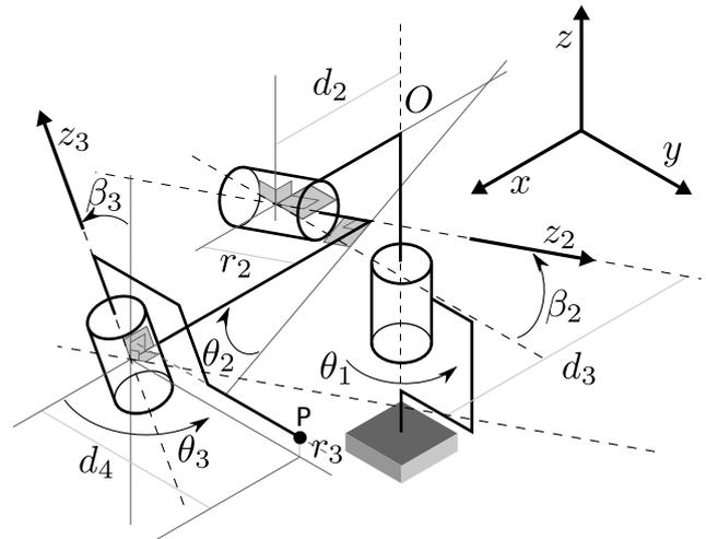
Figure 1. Kinematic diagram of a general 3R manipulator with  $\theta_1 = 0$ .
