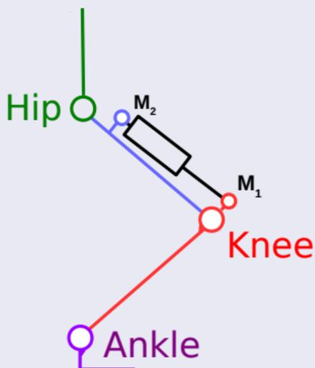
Figure: The single actuator architecture studied for this preliminary work (left).
