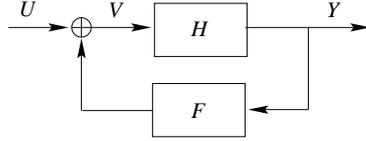
Figure 1: System  $H$  with an output feedback  $F$
