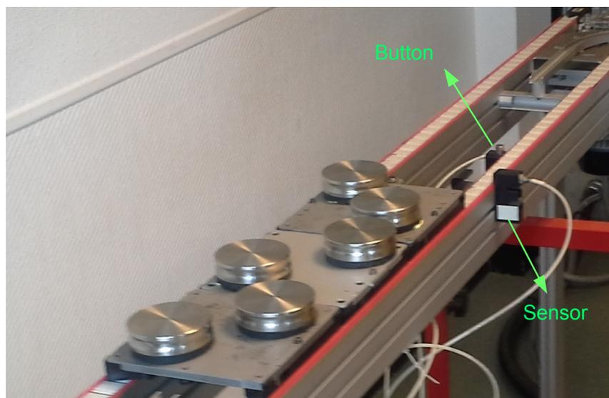
Figure 6.2: Three pallets in a line, approaching a button. When the button “fires” once, only one pallet continues moving and the other two continue waiting for another firing of the button.
