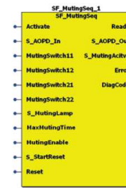
Fig. 53: Function block for sequential muting
