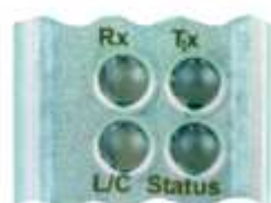
Fig. 62: Status LEDs of an ETHERNET Powerlink interface
