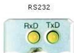
Fig. 61: Status LEDs for an RS232 interface
