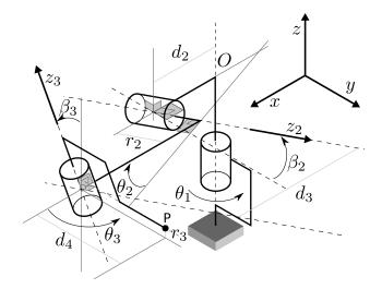
Figure 1. Kinematic diagram of a general 3R manipulator with  $\theta_1=0$ .
