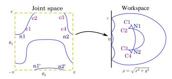
Figure 2. Singular sets in the space of the last two joints  $(\theta_2, \theta_3)$  and in the cross section  $(\rho = \sqrt{x^2 + y^2}, z)$  of the workspace, for a 3R orthogonal manipulator with parameters  $d_2 = 1$ ,  $d_3 = 1.5$ ,  $d_4 = 0.7$ ,  $r_2 = 0.5$ ,  $r_3 = 0.5$ .
