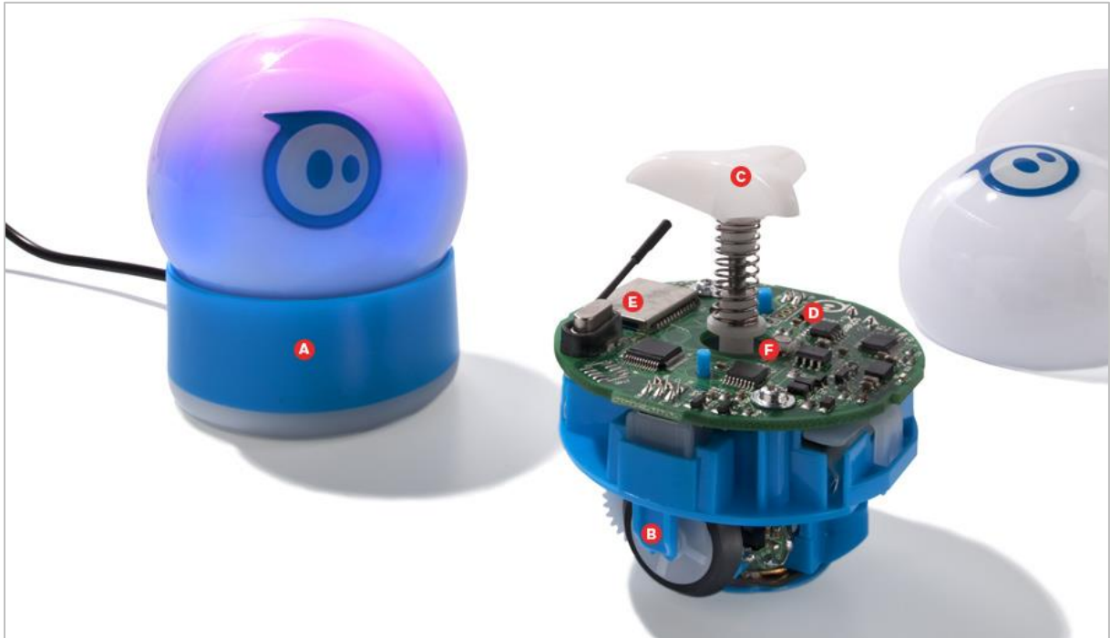
Figure 1: Composition du robot Sphero (Source : technologyreview.com )
