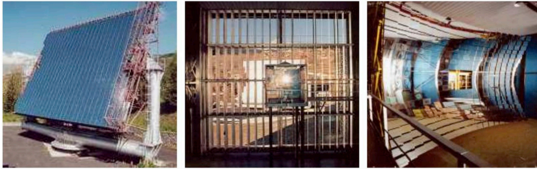
Fig. 3. Main Solar Furnace (reflector, modulator, concentrator).
