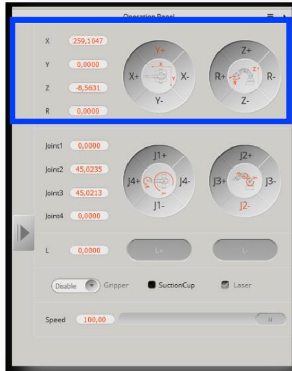
Figure 11: Setting in motion, in the + or - direction, along the X, Y, Z axes of the reference frame of the robot arm, or around the R axis.
