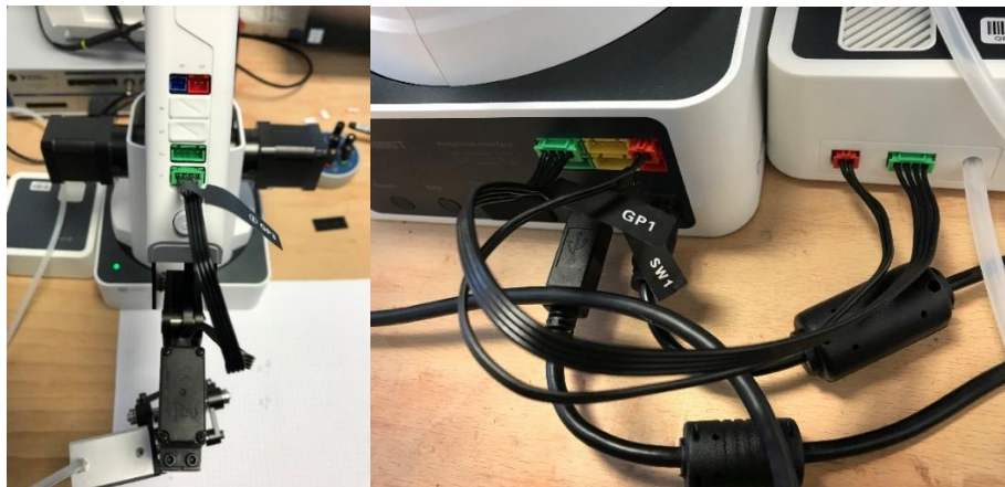
Figure 22: Connecting the gripper and mini-compressor to the robot arm.
