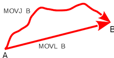
Figure 12 : Instructions MOVJ B, MOVL B.
