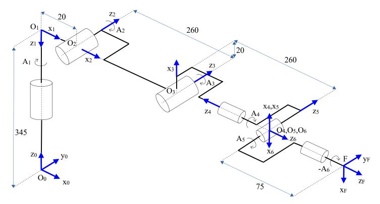
$R_0$  is the fixed reference frame (attached to the robot base),  $R_F$  is the frame attached to the robot flange (the coordinates of *F* are situated at the centre of the flange).
